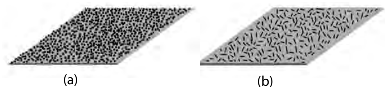
Figure 6.2 The diagram of uniform absorber distribution: (a) the cross-sectional view of equality distribution of particulate absorbers and (b) the cross-sectional view of equality distribution of fiber absorbers.
