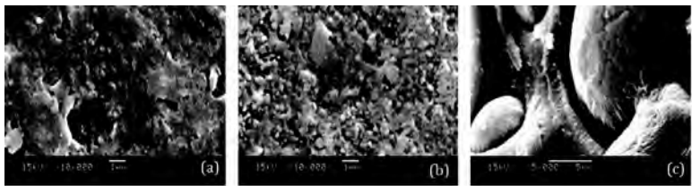
Figure 6.45 SEM images of nmCIP-reinforced composite coating sections: (a) nmCIP, (b) CB+nmCIP, and (c) FSA+nmCIP.
